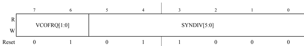
Figure 8-5. S12CPMU_UHV_V7 Synthesizer Register (CPMUSYNR)
