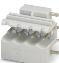
PCB headers, nominal cross section: 2.5 mm<sup>2</sup>, color: light gray, nominal current: 12 A, rated voltage (III/2): 320 V, contact surface: Sn, contact connection type: Pin, number of rows: 1, number of positions: 4, product range: MSTBO 2,5/..-G1R, connection method: pluggable, mounting: Wave soldering, number of solder pins per potential: 1, plug-in system: COMBICON MSTB 2,5, Pin connector pattern alignment: Orthogonal, locking: without, Product with pin output on right side
