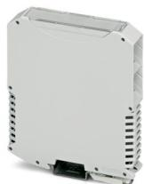
DIN rail housing, Complete housing with metal foot catch, tall design, with vents, width: 22.6 mm, height: 99 mm, depth: 113.65 mm, color: light gray (similar RAL 7035), cross connection: DIN rail bus connector (optional), number of positions cross connector: 5
