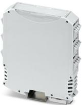
DIN rail housing, for mounting on a DIN rail, color: light gray (similar RAL 7035), width: 22.5 mm, height: 99 mm, depth: 113.65 mm, incl. 6 PCB connectors, 4-pos., screw connection, for 2.5 mm<sup>2</sup>, nominal current: 12 A, 320 V, PCB surface: 6800 mm<sup>2</sup>
