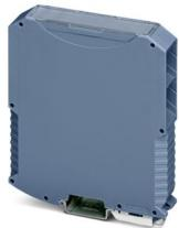
DIN rail housing, Complete housing with metal foot catch, tall design, without vents, width: 22.6 mm, height: 99 mm, depth: 113.65 mm, color: blue grey (similar RAL 7031), cross connection: DIN rail bus connector (optional), number of positions cross connector: 5
