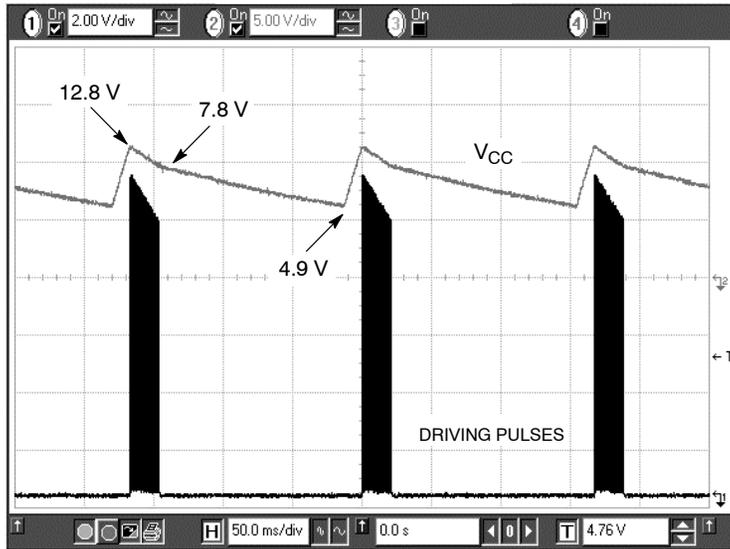
Figure 15. Typical Waveforms in Short Circuit Conditions
