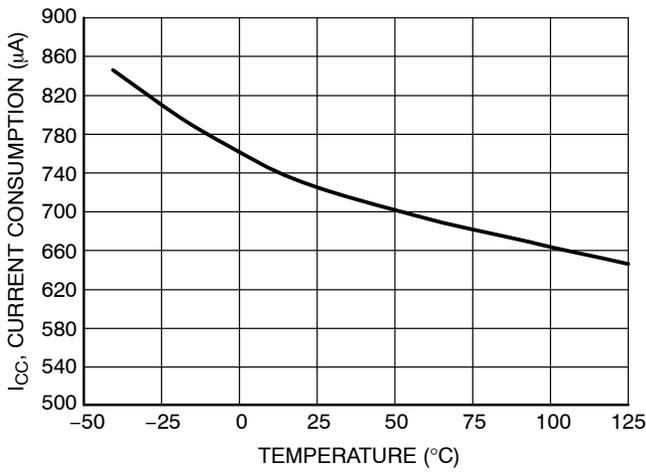
**Figure 5. I<sub>CC</sub> Current Consumption (No Load) versus Temperature**
