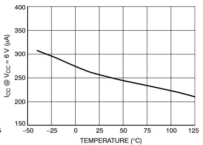
**Figure 8. I<sub>CC</sub> Consumption at V<sub>CC</sub> = 6 V versus Temperature**
