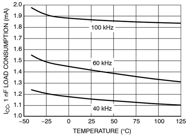
**Figure 6. I<sub>CC</sub> Consumption (Loaded by 1 nF) versus Temperature**
