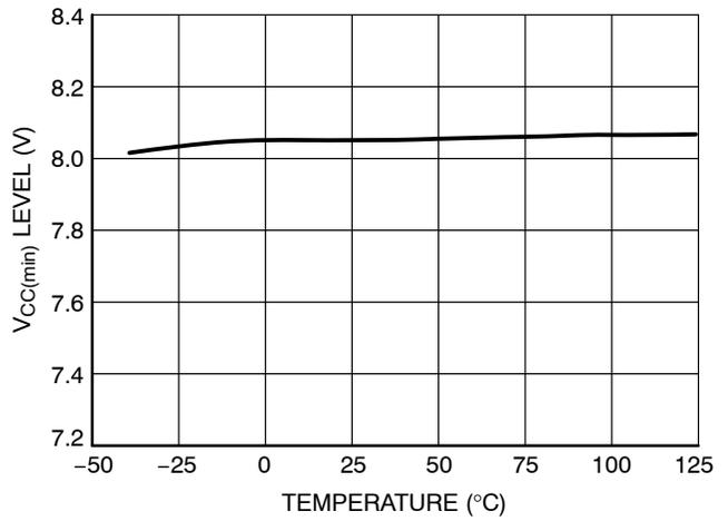
**Figure 4. V<sub>CC(min)</sub> Level versus Temperature**
