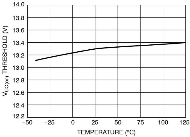
**Figure 3. V<sub>CC(on)</sub> Threshold versus Temperature**
