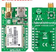
GPS Click - L10 is an accessory board in mikroBus<sup>TM</sup> form factor. It's a compact solution for adding GPS functionality to your device. It features **Quectel® L10**, high performance MTK positioning engine. GPS Click - L10 communicates with target board through UART or I<sup>2</sup>C interface. Data can be acquired using PC application through USB connection. Board features connector compatible with active and passive antennas. It can operate on 3.3V power supply only.
