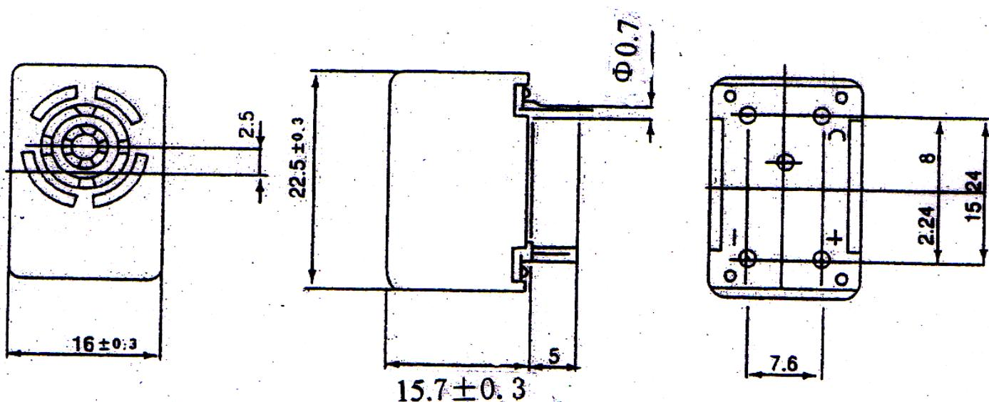
**Must connect “-“ to ground; “+” & “C” to positive voltage for operation.**
