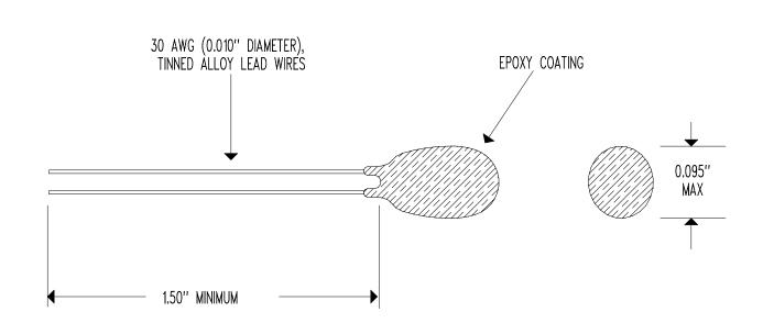
RESISTANCE @  $+25^{\circ}C$  =  $100,000 \Omega$  NOMINAL ACCURACY (0 TO  $+70^{\circ}C$ ) =  $\pm$  0.20°C RESISTANCE/TEMPERATURE CURVE = "J" TEMPERATURE COEFFICIENT @  $+25^{\circ}C$  = -4.4%/°C NOMINAL BETA " $\beta$ " (0 TO  $+50^{\circ}C$ ) =  $3,892^{\circ}K$  NOMINAL DISSIPATION CONSTANT = 1 mW/°C NOMINAL THERMAL TIME CONSTANT = 10 SECONDS MAXIMUM (STILL AIR) THERMAL TIME CONSTANT = 1 SECOND MAXIMUM (WELL STIRRED OIL) MAXIMUM TEMPERATURE RATING =  $+150^{\circ}C$
